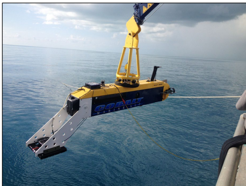
Dolores HAUV being deployed with EM system attached
